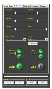
In the right hand column of sliders you can adjust the **Brightness** and **Contrast**. Typically you will leave these in the center. **Power** controls the probe's pulse power. Typically, **Power** will be at the maximum unless the image is saturated with the **Gains** centered.
