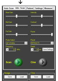
In the right hand column of sliders you can adjust the **Intensity** and **Contrast**. Typically you will leave these in the center. **Power** controls the probe's pulse power. Typically, **Power** will be at the maximum unless the image is saturated with the **Gains** centered.
